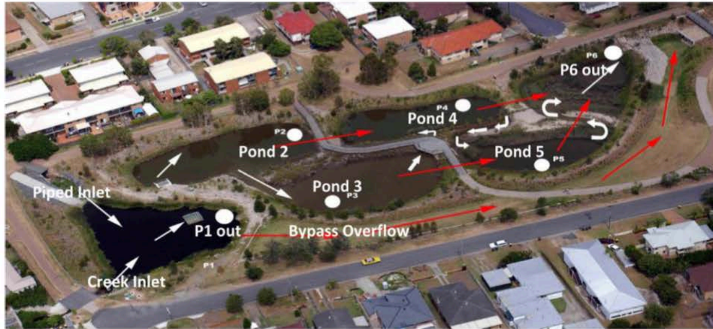
Fig. 2. Aerial view of the Bridgwater Creek constructed wetland system: Bowie's Flat Wetland showing sampling sites (P1out:Pond1-sediment basin; P2: Pond2; P3:Pond3; P4:Pond4; P5:Pond5; P6out:Pond6). The white arrows depict base flow and stormwater flow during 'average rainfall' events. The red arrows depict stormwater flow during 'high intensity rainfall' events. (For interpretation of the references to colour in this figure legend, the reader is referred to the web version of this article.)
